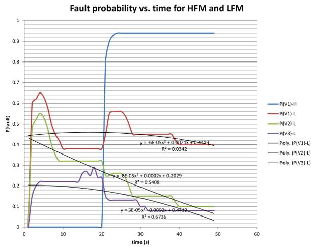
Figure 6: Diagnosis probabilities computed for an LFM, with fault injection at time  $t = 20$ , with  $2^{nd}$  order polynomial correction factors
