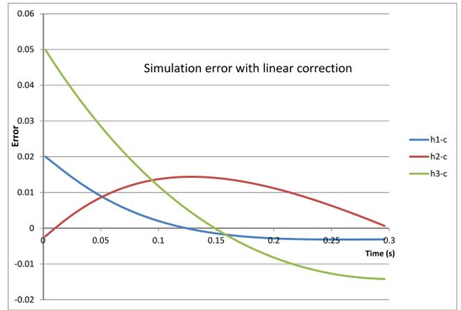
Figure 4: Corrected LFM simulation of tank benchmark, using linear linking function, with initial condition of  $h_1(0) = 1$ ,  $q_0 = 1.5$ .
