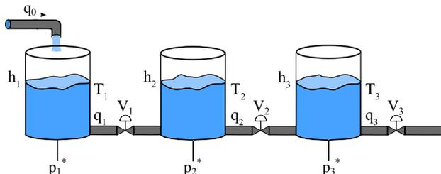
Figure 1: Diagram of the three-tank system.
