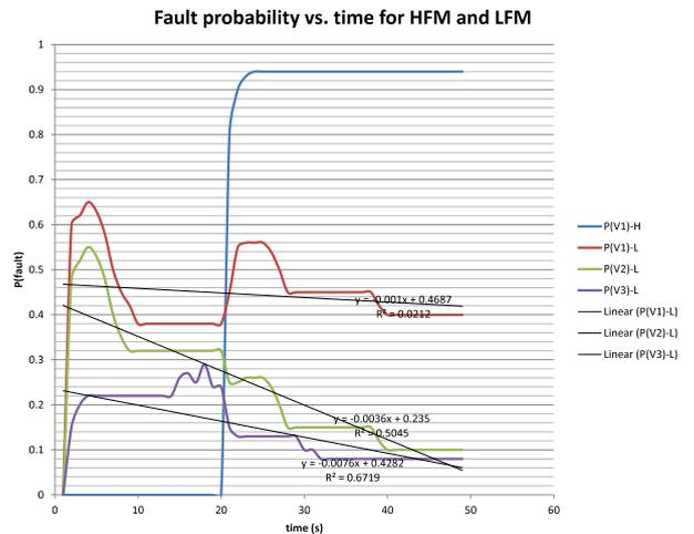
Figure 5: Diagnosis probabilities computed with fault injection at time  $t = 20$ , with linear correction factors.  $P(V_1)$ -H denotes the HFM data, and  $P(\cdot)$ -L denotes the LFM data.
