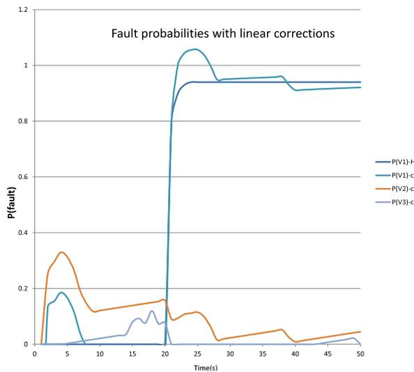
Figure 7: Corrected LFM Diagnosis probabilities, with fault injection at time  $t = 20$
