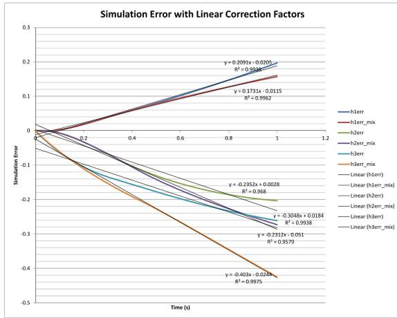
Figure 3: Relative error of simulation of tank benchmark with initial condition of  $h_1(0) = 1$ ,  $q_0 = 1.5$ . Data shows results for linear model plus a mixed model containing a partial linearization: for example, h1-err and h1-error-mix shows the error is height of tank 1, for the linear and mixed models respectively. Linear- denotes the form of the linear correction factor, together with its  $R^2$  fit.
